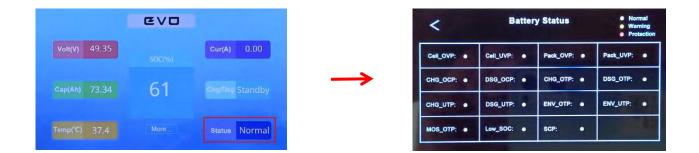
(4) Click "**More**" to view the battery information include the Battery Voltage & Temp. Cell 01 to Cell 15 voltage, T1 to T4 temperature, T\_MOS,T\_ENV.
