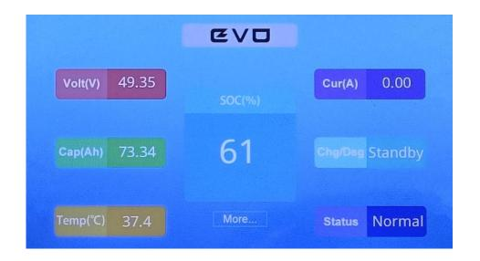
(2) Click **"Volt(V)**" to read the battery information include Voltage, Current, Status, SOC, Vmax, Vmin,RMC, FCC,Warn, Protect, Tmax, Tmin.
